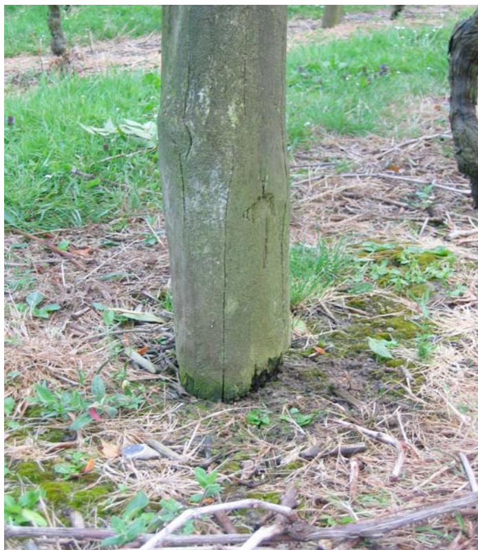
Picture: 10-12 year old wood post rotting at its base in poorly drained clay soil
